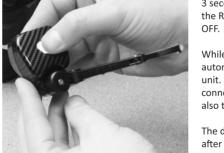
TURNING THE MAIN UNIT OFF To turn the device OFF, press the button on the MAIN unit and hold it for approx. 3 seconds until the LED turns RED. When the RED light turns off, the MAIN unit is
